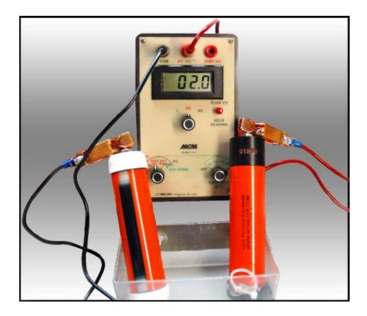
Since the IonX electrode potential was quoted as 318mV versus SHE on its Calibration Certificate, and, since the voltmeter reading (potential difference reading) was indicated as 2mV (see the LCD in the above photograph), the electrode potential of the RE-5C electrode, in this example, would be inferred to be 316mV versus SHE (318mV plus 2mV).
