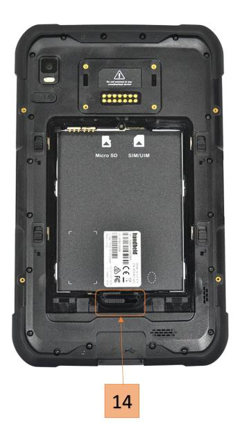
With the battery cover off, locate the battery latch (#14) and slide to the left to unlock. The battery can then be removed by turning the tablet over and GENTLY tapping it against the palm of your hand.
