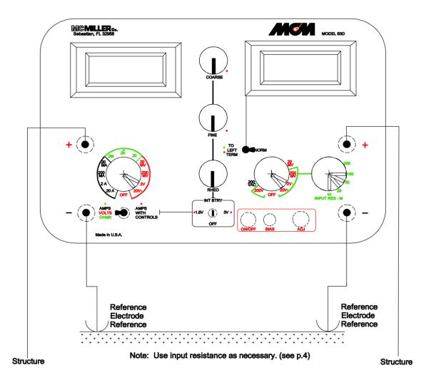
Use of internal controls to control current from an external battery or other source of current.
