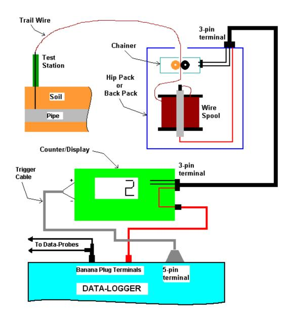
Figure 2: Counter/Display Unit Mounted on Tray – Connections for Automatic Triggering of Readings
