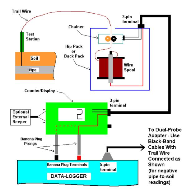
Figure 3: Counter/Display Unit Mounted Directly on Data-Logger - Connections for Manual Triggering of Readings Using Data-Probe Push-Buttons
