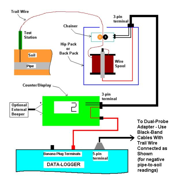
Figure 1: Counter/Display Unit Mounted on Tray – Connections for Manual Triggering of Readings Using Data-Probe Push-Buttons
