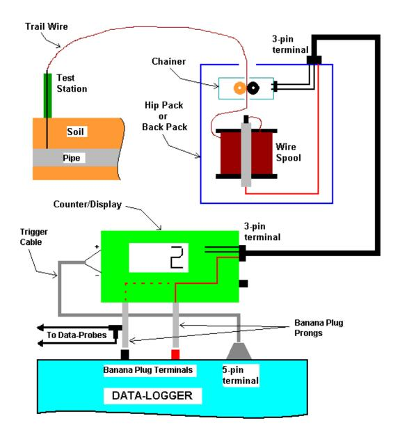
Figure 4: Counter/Display Unit Mounted Directly on Data-Logger Connections for Automatic Triggering of Readings
